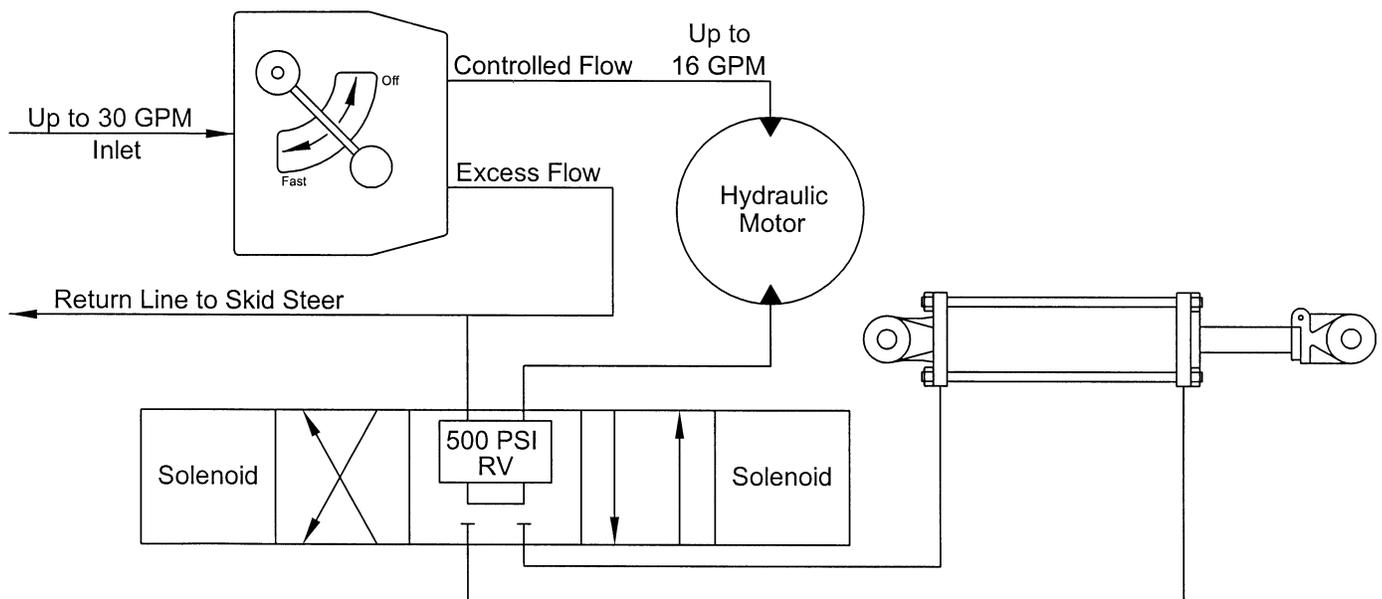
Figure 9 – Schematic of Solenoid Valve Hydraulic Connections
