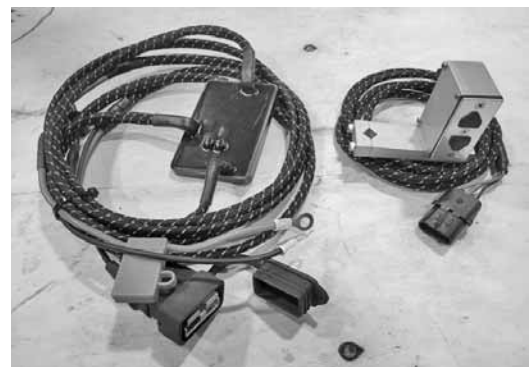
2507038 – Complete Wiring Harness (Combined 2507036, 2505844 & 2507037)
