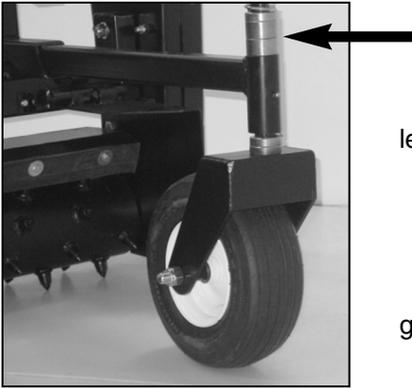
Posi-Lock wheel spacers allow the adjustment of the gauge wheels for proper leveling of the machine, which determines the rotor cutting depth.
