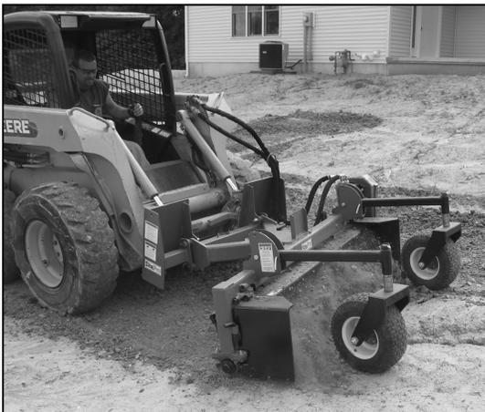
**NOTICE:** When angling the power rake, there could be side pull (rotor walking in the direction the power is directed and rotation of rotor). Operator must be aware of this and steer the prime mover to stay in the intended direction.
