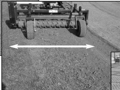
**Blending existing and processed lawn together:** Set gauge wheels on one side of the machine, let 6" up to 12" of rotor over hang the existing lawn. Out side rotor tooth will be either just touching or not touching surface, while other side will be touching and processing the material to bring the two surfaces together.
