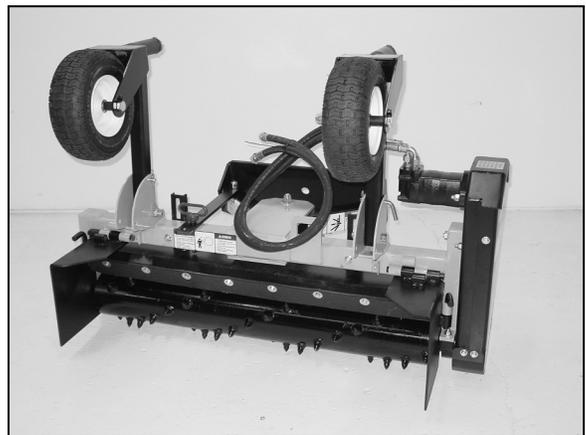
To flip-up the gauge wheels, take some pressure off the wheels by lifting the unit up slightly. Remove the pin and raise the wheel assembly to the upright position. Install the pin in the upper hinge plate hole and thru the gauge wheel arm to lock it in place. Replace the clip in the end of the pin.
