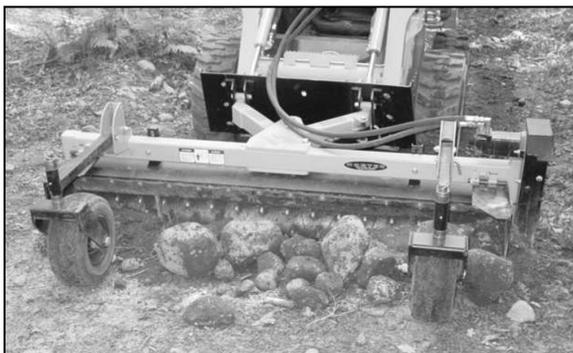
Once the surface has been loosened, the process of removing debris can begin. The prime mover attachment plate is tilted forward until the guide wheels control the depth of the toothed rotor. The rotor can be angled at this time for windrowing debris or the rotor can be set straight with both side shields down to collect debris. Prime mover travel speed can be increased for this process.
