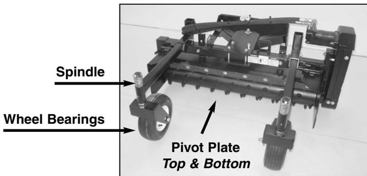
**NOTICE:** Pivot greasing is VERY important. If not properly greased and maintained, manual angle will be very hard if not impossible to turn. Make sure to grease both top and bottom grease fittings. After greasing pivot frame left and right several times to smear grease on pivot plate.
