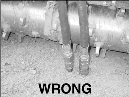
Keep hydraulic fittings off the ground to prevent damage and collecting dirt and foreign material.
