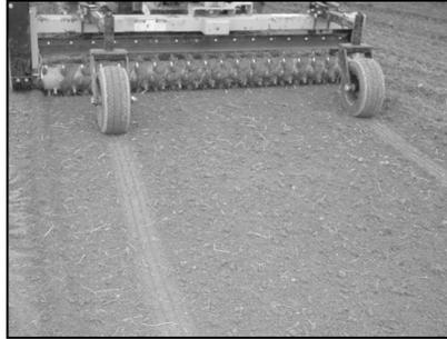
**Final Grade:** Set the rotor teeth so they are just touching the surface. This will collect the small rock and debris. This is where the raking action occurs not the processing action. (see note)
