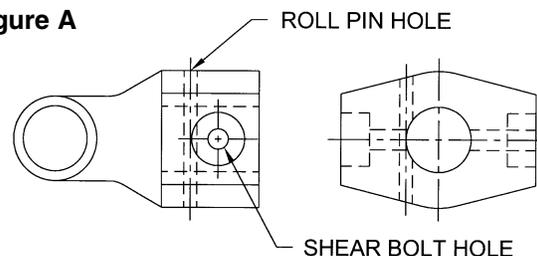
On the implement end of the PTO shaft there is a hole in the yoke just forward of the 3/8" shear bolt (see Figure A). This hole is for the 1/4" diameter x 2 1/4" long roll pin (Ref. #20). When this roll pin is driven in this hole, the center of the roll pin engages into the groove on the front of the gearbox input shaft. This prevents the PTO assembly from coming off if the 3/8" shear bolt should shear.
