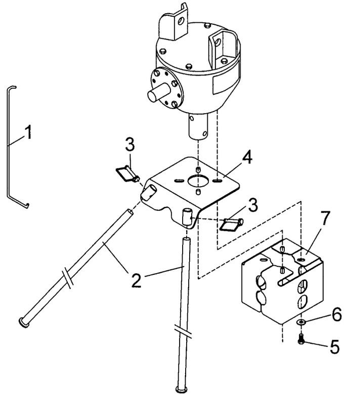
The Parking Stand Kit has a plate that bolts to the bottom of the gearbox. Two removable legs go into sockets welded on the plate. The legs are pinned in place. The two legs and the auger form a tripod which supports the post hole digger in a vertical position. A formed hook keeps the PTO driveline end off the ground.
