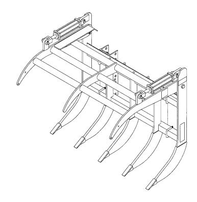
Grapple Rake for Skid Steer and Tractor Front Loader
