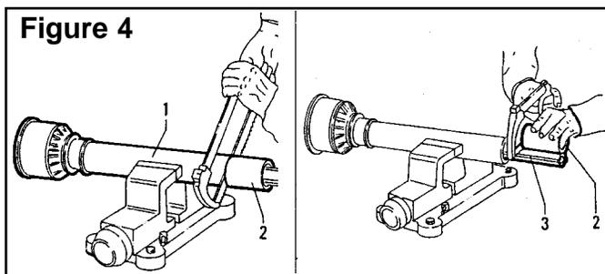
4. If driveline must be cut to a shorter length, clamp driveline in a well padded vise to prevent damage to the shield. Cut off shield where marked. Using cut-off section of shield as a guide, cut shaft the same amount. (Figure 4.)
