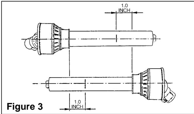
1. Place the two halves of the driveline together, keeping them parallel (see Figure 3). Using a felt-tip pen, matchmark the place where the two halves must be shortened, measuring 1.0 inch from the beginning of each half, as shown in Figure 3.
