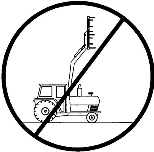
Keep the Bale Handler as low as practical at all time to reduce the possibility of tipping or contacting overhead obstructions. Braking efficiency will also be less if the center of gravity is raised.
