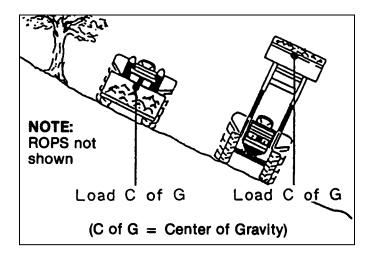
When working on side hills, **DO NOT RAISE LOADER TOO HIGH.** Keep an eye on terrain changes. Keep load low.
